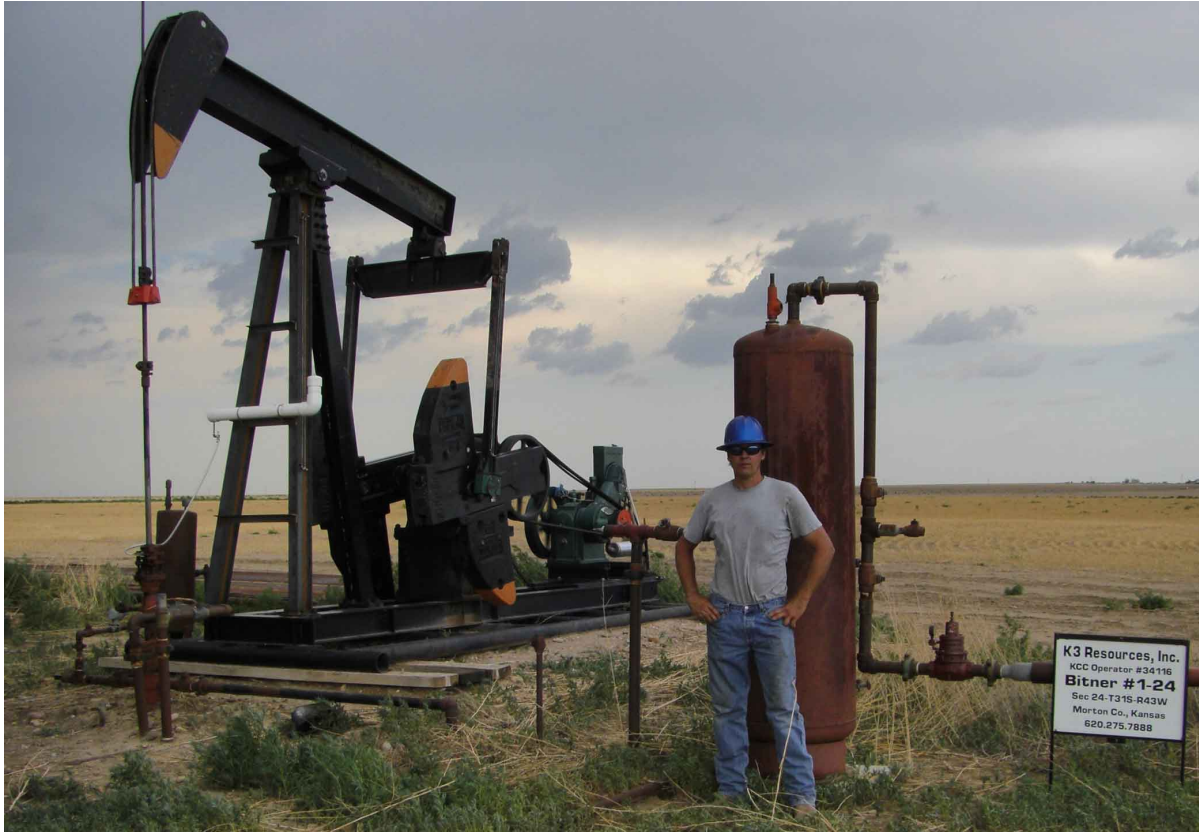
Figure 1 – A typical field location showing a pumping unit and surface plumbing used to deliver gas or oil to the sales pipeline. Digital instrumentation can be used to relay operational data to a remote monitoring workstation.
