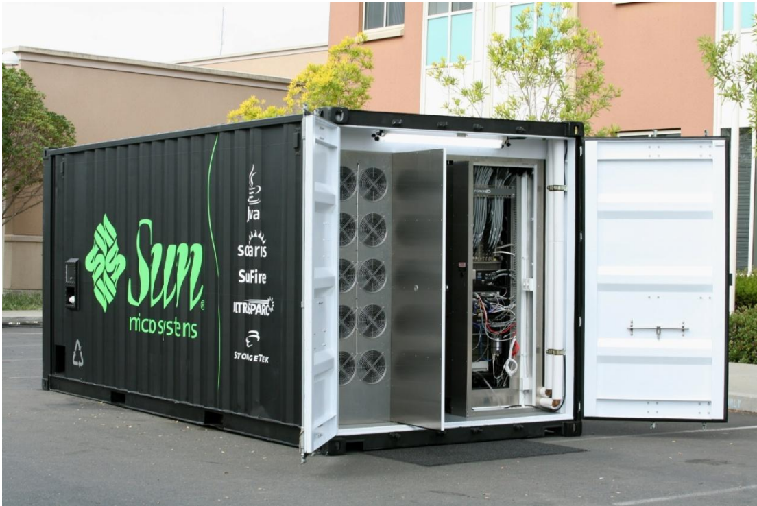
Figure 9 – A modular container filled with server computers is typical of the data centers powering Google, Amazon, and Facebook.
